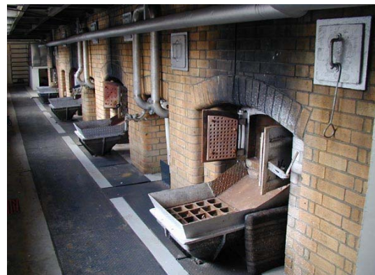
The old coal-fired furnaces in distillery
